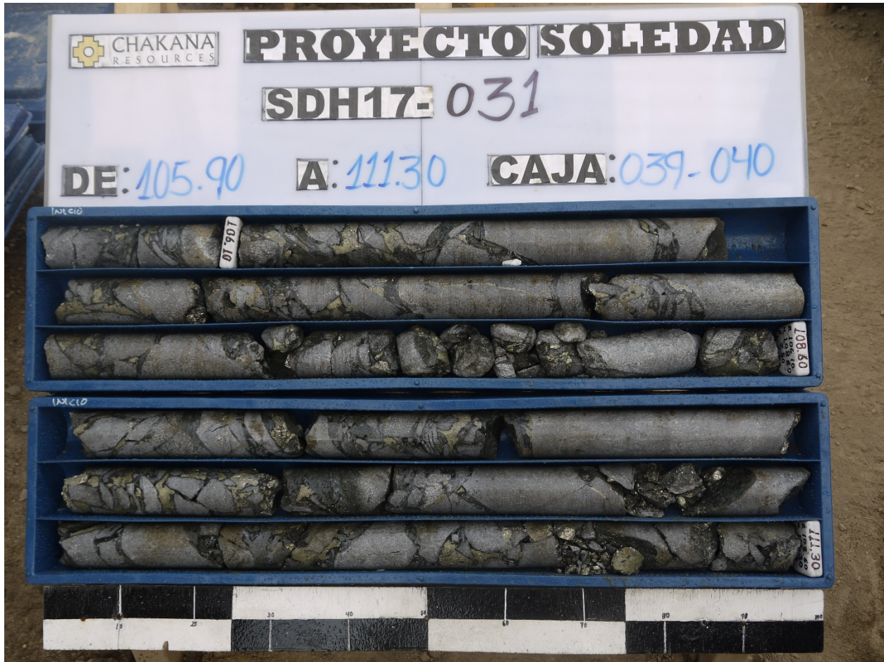
Figure 1 – Core from SDH17-031 for 105.9 to 111.3m showing strong copper mineralization in the matrix of the tourmaline breccia.
