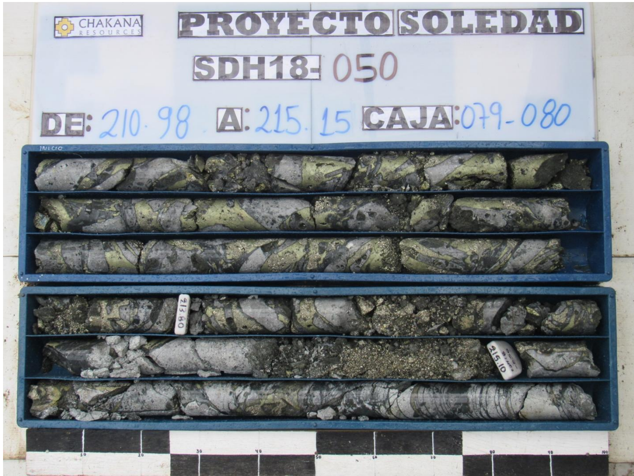
Figure 1 – High grade margin zone mineralization from hole SDG18-050 in Bx 1. The five metre interval from 210.00-215.00 averages 8.15% Cu, 2.22 g/t Au, and 94.2 g/t Ag.
